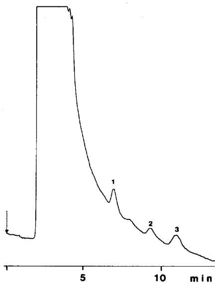
Fig. 3. Chromatogram obtained by concentrating 1000 ml of tap water spiked with 0.1 \mu\text{g/l} of dicamba (peak 1), 0.1 \mu\text{g/l} of 2,4-D (peak 2) and 0.2 \mu\text{g/l} of bentazon (peak 3) using a PRP-1 cartridge. Mobile phase: acetonitrile–water (40:60), pH 2.
